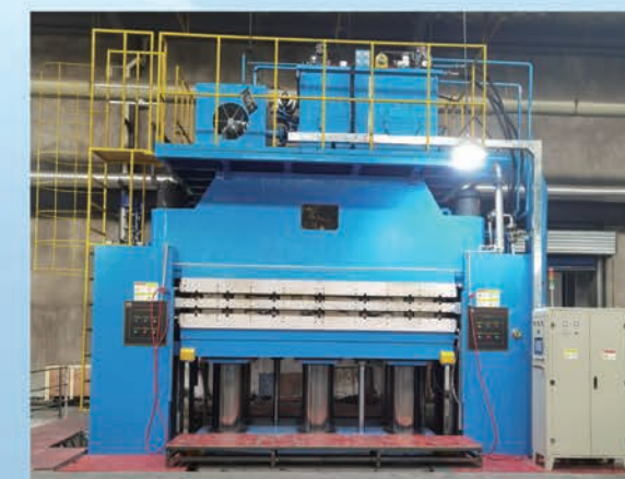
Sealing ring vulcanizer for plate heat exchanger
