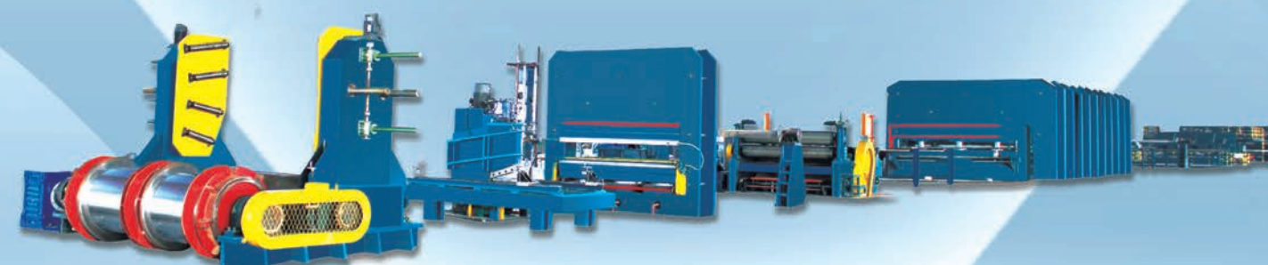
Equipment of 2800×16600/210.00MN wire rope production line
