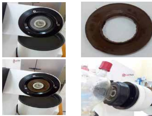
Figure 8. Photograph of sealers made by the NR/NBR/silica composites and its uses
