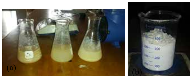
Figure 1. Photograph of (a) silica gel and (b) Purified silica
