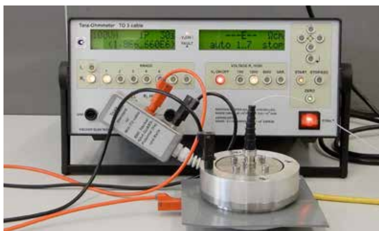
Figure 1. A sample of rubber containing TUBALL™ MATRIX 618 beta having its volume resistivity measured according to ASTM D257.
